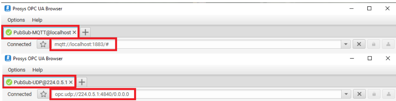
Figure 37. The title and address bar are named to describe the PubSub connection and subscription.
