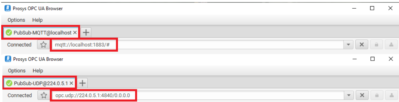
Figure 43. The title and address bar are named to describe the PubSub connection and subscription.
