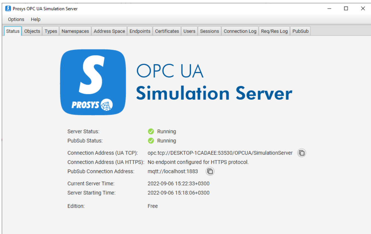
Figure 2. The Status View displays some basic information about the server and PubSub connection.
